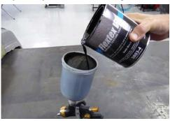
9. Apply Flextex VT in light "splatter" coats from a distance of about 16 inches (40 cm) from the bumper. Move gun quickly to keep texture even and to avoid flowing out the paint. Allow five minutes of flash time between coats. Apply at least three coats to achieve desired textured appearance.
