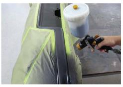
Sand with 240-320 grit sandpaper to remove underlying sandscratches. Fill imperfections with spot putty. Spray a second coat of 3043 Black Jack, dry, and sand again with 320. Achieve a smooth primered surface prior to application of Flextex VT.
