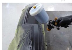
May be used without top coating or top coat with base/matte clear or hardened basecoat any time after completely dry.
